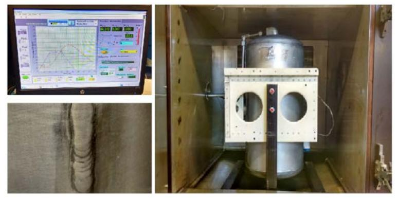
Fatigue Testing is carried out with the objective of determining the relationship between the stress range and the number of times it can be applied before causing failure.
